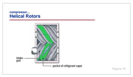
The entering refrigerant vapor is at a low, suction pressure and fills the grooves or pockets formed by the lobes of the rotors. As the rotors turn, they push the pockets of refrigerant toward the discharge end of the compressor.
